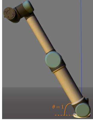
Figure 4.3: Screenshot from visualization of robotic arm. For simplicity, the relative angles of all joints except the first one is set to 0.0. Source publication 10
